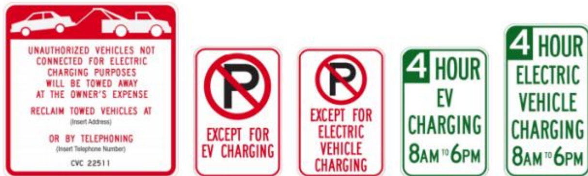
Figure 14: Examples of parking signs to place restrictions or time limits on charging spaces
